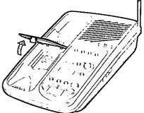
Install the battery in the battery compartment.
