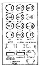
If the SCREEN/PLAYBACK indicator flashes when you press SCREEN/PLAYBACK or "#", the answering system is off. To turn it on, press "8".
