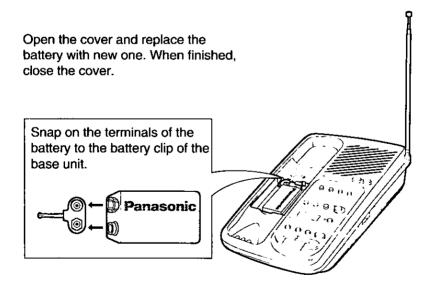
• See page 10 for details of installing the 9V (6F22) size battery.
